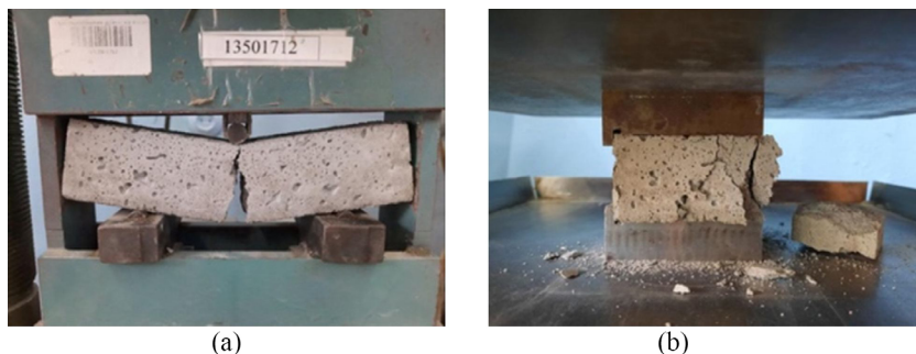
Fig. 12. The process of testing beam samples: (a) flexural strength; (b) compressive strength
