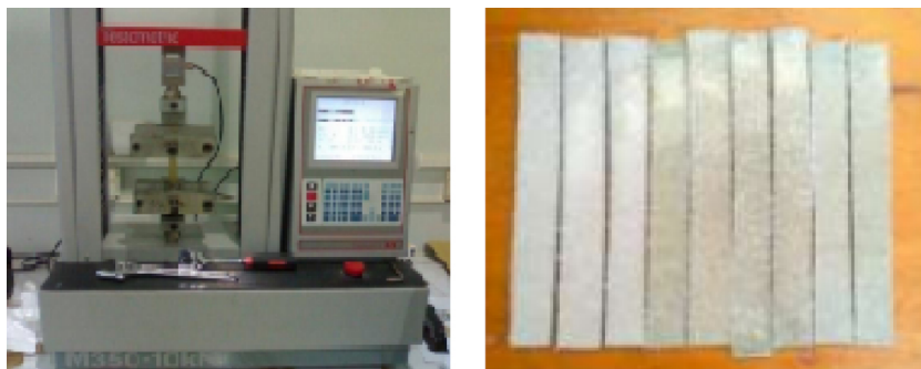
Fig. 3. Tensile testing machine and test samples
