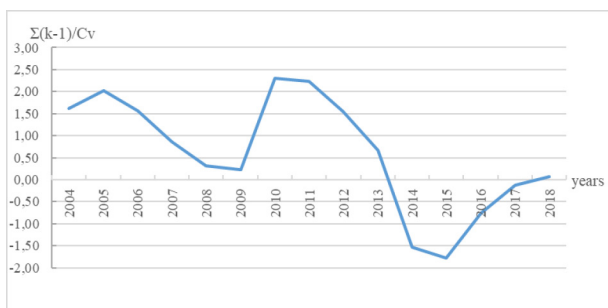
Fig. 3. Difference integral curve of average annual water consumption of the Charyn River, Sarytugay tract, for 2004–2018
