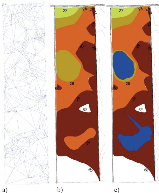
Fig. 1. a – triangulation of the surface, b – digital model digital model of the relief of the studied area, c – hydrodynamic model of flooding of the area of the studied area
